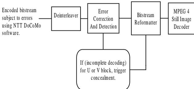
Figure 2: Proposed Decoding Scheme
